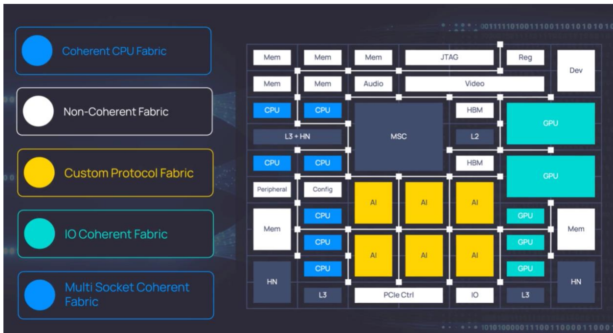
Figure 1: A Unified Fabric across a SoC links the various NoCs with a single transport layer.
